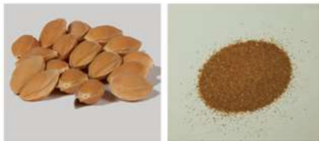
Fig. 1. Apricot stone shell used as reinforcing element
